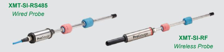
ProGauge Magnetostrictive Level probes provide continuous and highly accurate readings of liquids inside of the tank. By transmitting a high frequency electrical impulse that travels at the speed of sound, the advanced technology within the probes is able to measure the time elapsed between the initial sending of the signal and its return to the float, giving an unbeatably accurate fuel reading which is then relayed to the ProGauge console on site or directly to the Point of Sale (POS).
